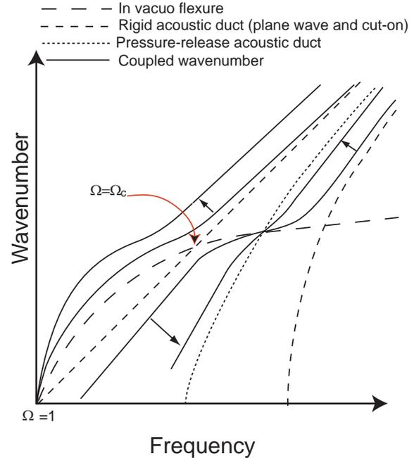
Figure 9: Schematic of the coupled wavenumber solutions. Arrows indicate the transition of solutions as  $\epsilon$  increases.
