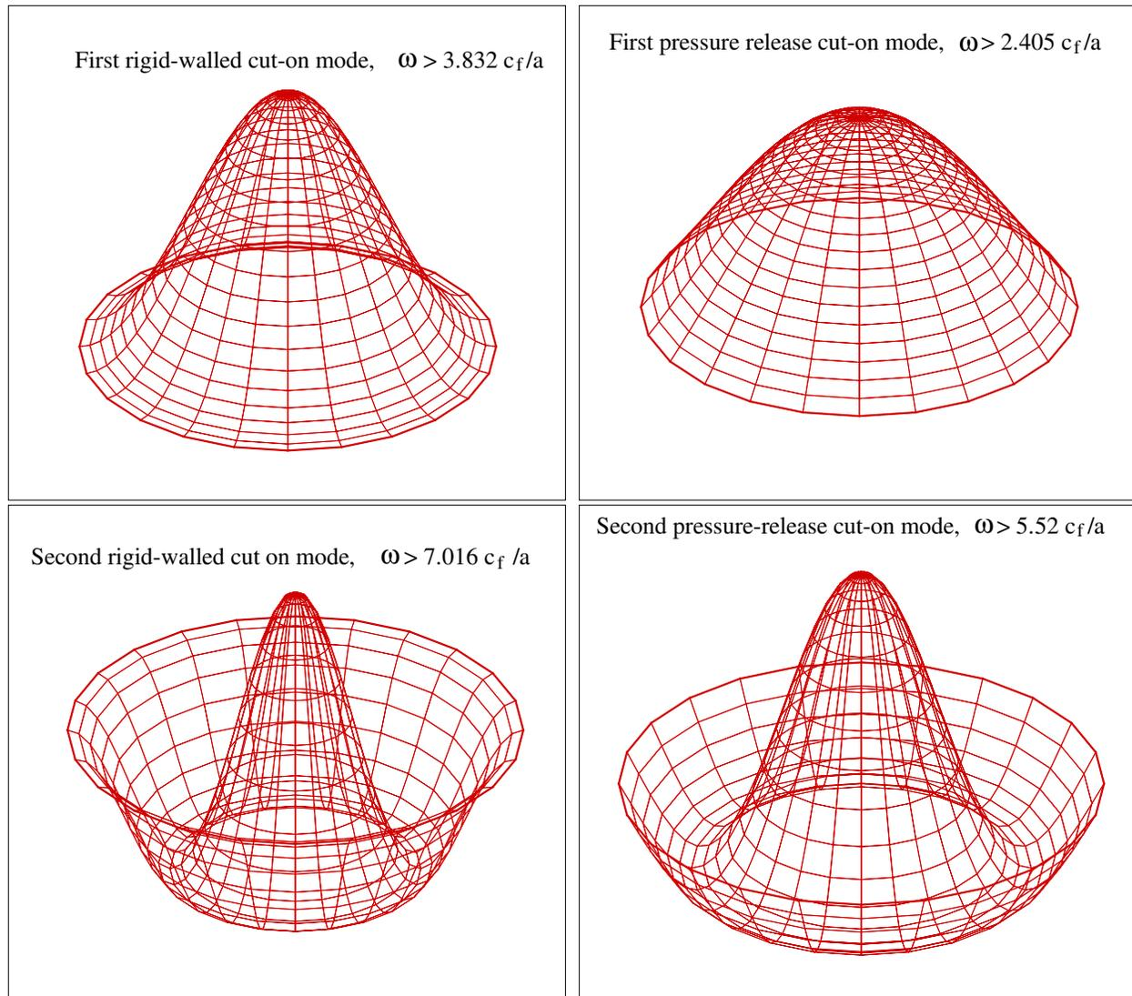
Figure 2: Cut-on acoustic modes in cylindrical duct for the axisymmetric mode ( $n = 0$ ).
