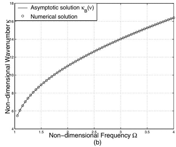
Figure 4: Wavenumber corresponding to the dominantly bending mode obtained through the asymptotic method and the numerical solution for  $\nu = 0.25$  and  $h/a = 0.05$ . (a) Below the ring frequency ( $\Omega < 1$ ) (b) Above the ring frequency ( $\Omega > 1$ ).
