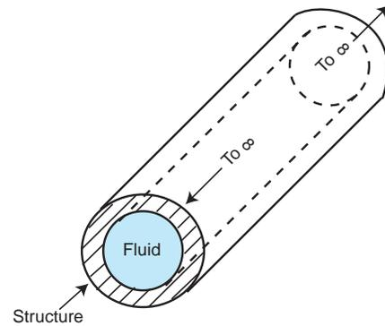
Figure 1: Schematic of the model showing the fluid-filled flexible cylindrical shell of infinite length.
