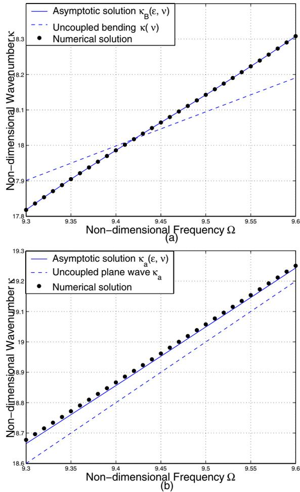
Figure 8: Coupled wavenumber solution above the coincidence frequency ( $\Omega_c$ ) for the fluid-filled infinite cylindrical shell with  $h/a=0.1$ ,  $c_L/c_f=2$ ,  $\epsilon=0.2$  and  $\nu = 0.25$ , vibrating in the axisymmetric mode (a) for the bending wave (b) for the acoustic plane wave.
