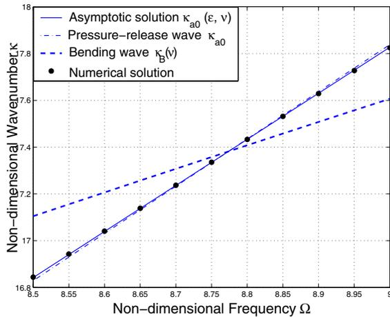
Figure 5: Coupled wavenumber solution near the first acoustic pressure-release cut-on mode for  $h/a = 0.1$ ,  $c_L/c_f = 2$ ,  $\varepsilon = 1.25$  and  $v = 0.25$ .
