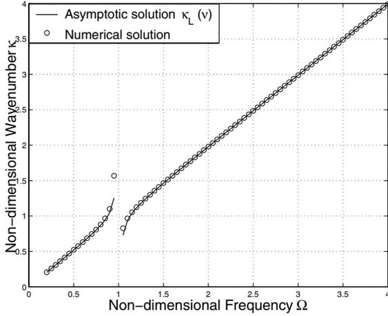
Figure 3: Wavenumber corresponding to the dominantly longitudinal mode obtained through the asymptotic method and the numerical solution for  $\nu = 0.25$  and  $h/a = 0.05$ .
