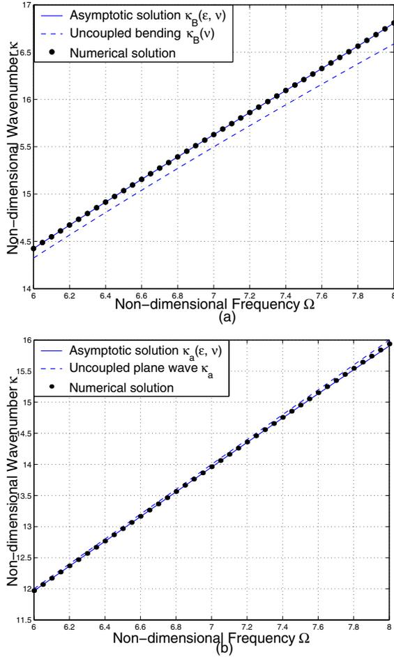
Figure 6: Coupled wavenumber solution below the coincidence frequency ( $\Omega_c$ ) for the fluid-filled infinite cylindrical shell with  $h/a=0.1$ ,  $c_L/c_f=2$ ,  $\varepsilon=0.2$  and  $\nu = 0.25$ , vibrating in the axisymmetric mode (a) for the bending wave (b) for the acoustic plane wave.
