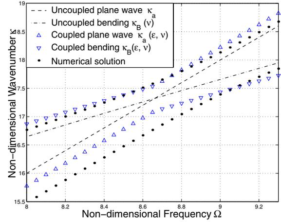
Figure 7: Coupled wavenumber solution near the coincidence frequency for the fluid-filled infinite cylindrical shell with  $h/a=0.1$ ,  $c_L/c_f=2$ ,  $\varepsilon=0.2$  and  $\nu = 0.25$ , vibrating in the axisymmetric mode.
