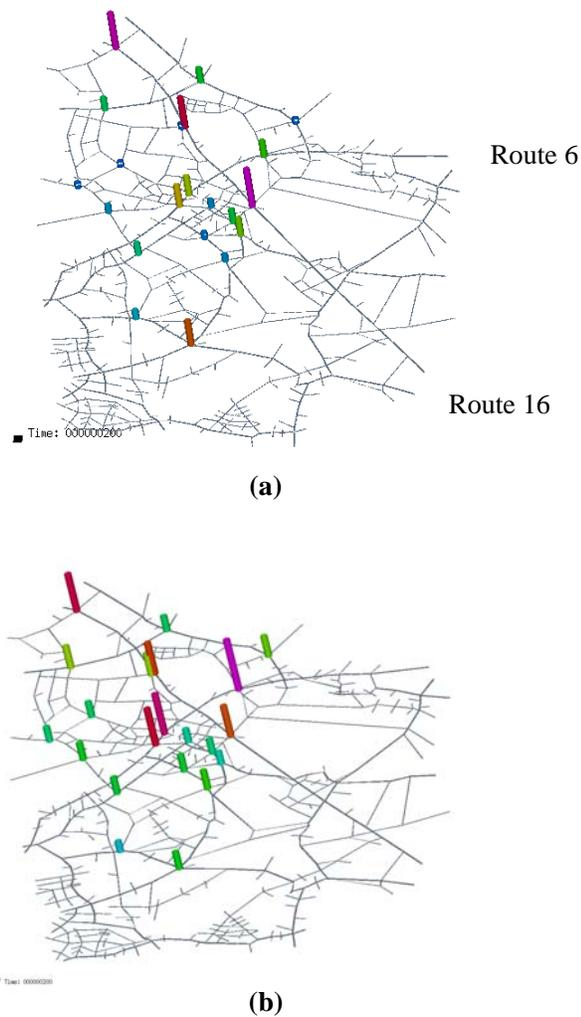
**Figure 8** : (a) Simulated result of traffic demand during 7-8AM at 21 intersections (b) Observed result of traffic demand during 7-8AM at 21 intersections
