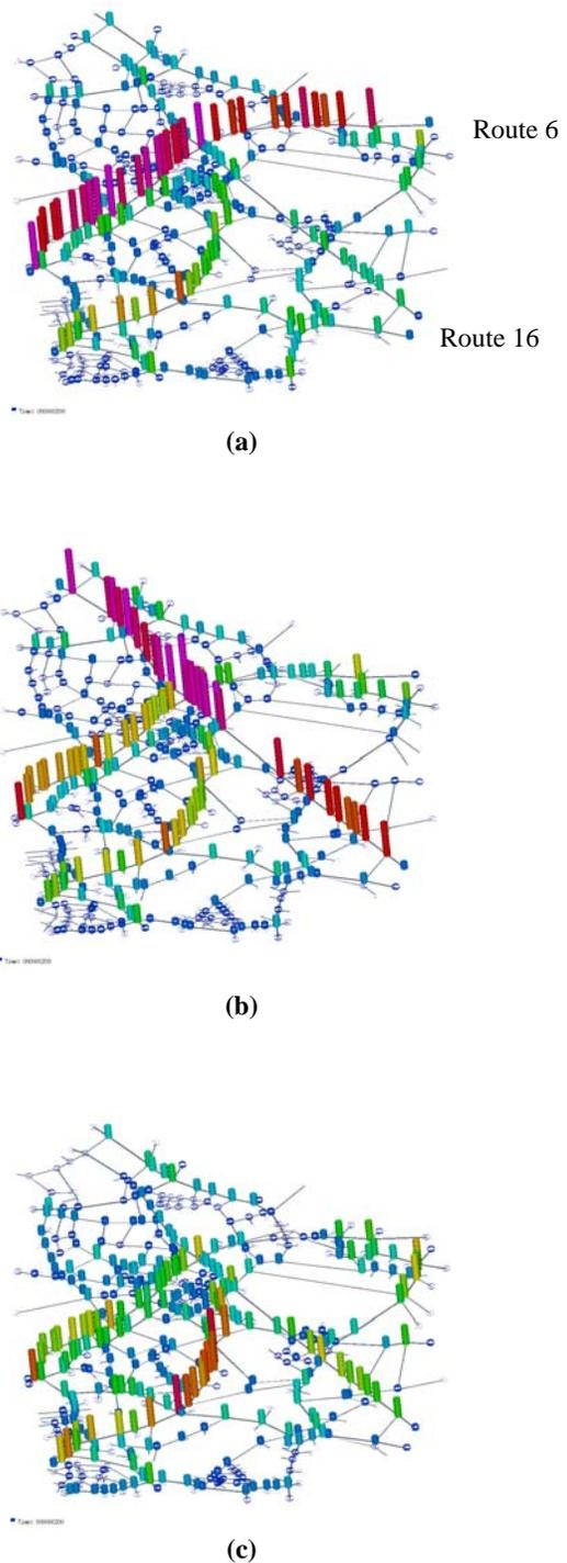
**Figure 7** : (a) Accumulated traffic demand for 30 min (Case 1); (b) Accumulated traffic demand for 30 min (Case 2); (c) : Accumulated traffic demand for 30 min (Case 3)
